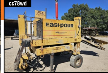
CURB AND GUTTER MACHINE
